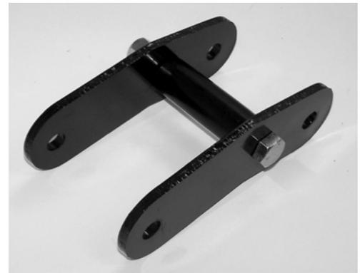
toward the front bumper. If installing on the rear of the vehicle the short end of the shackle should be facing the ground with the dogleg angled toward the rear bumper. The orientation of the shackle is very important due to clearance issues.
